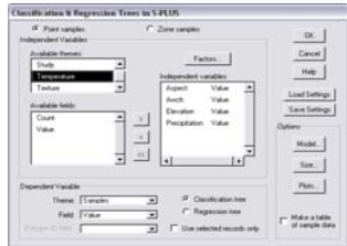
Figure 3. Classification & Regression Trees dialog box. In this example, the Value fields from the Aspect, Azch, Elevation, and Precipitation themes will be used as independent variables for a classification tree model. The dependent variable will be the Value field from the Samples point theme.
